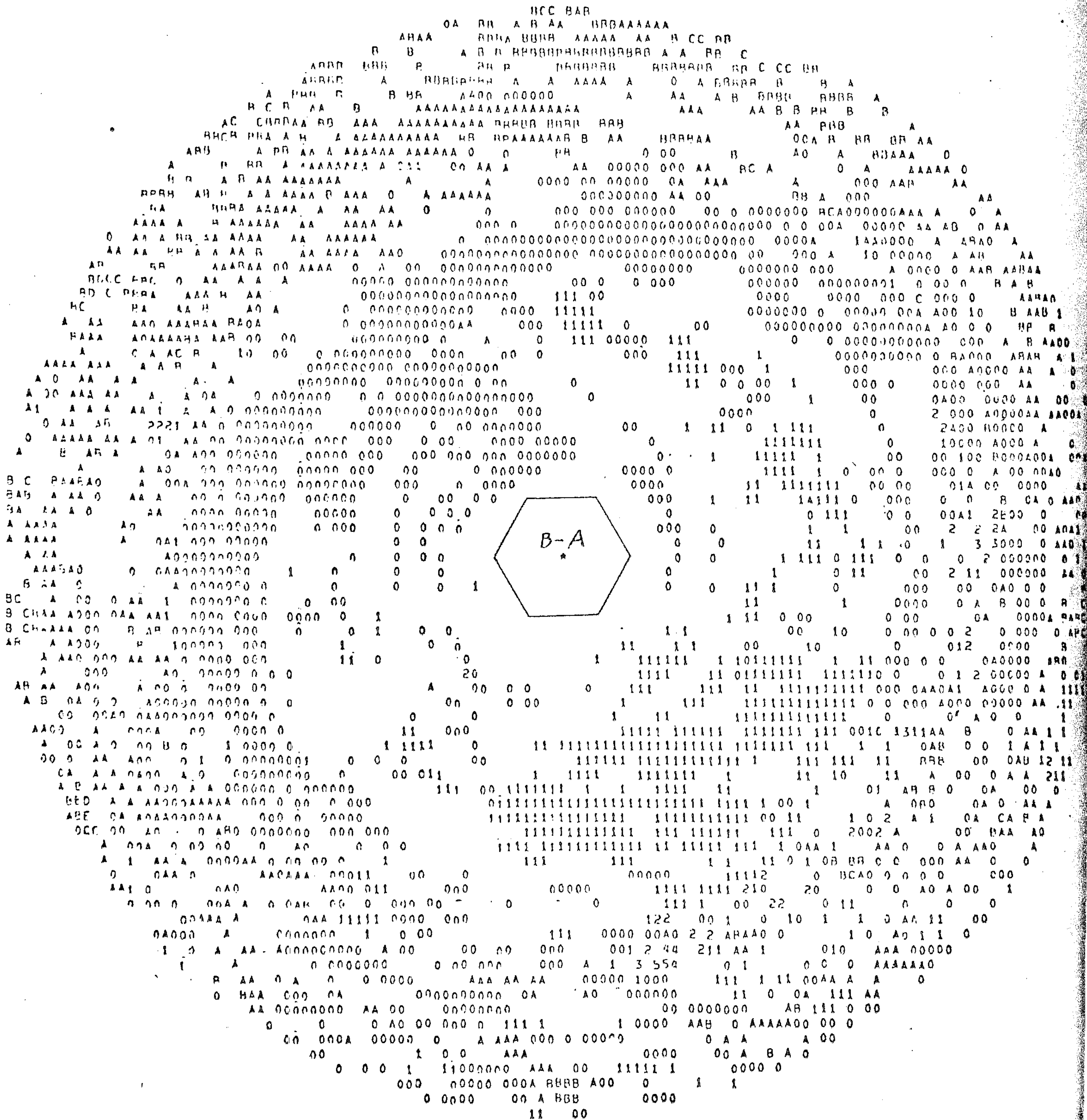
Figure 16: This figure is a plot of the point-by-point difference ( 1^\circ in azimuth, 7.5 cm radially) between two successive measurements of the prototype dish surface. One of the data sets is that of Fig. 15. The rms difference is 20 \mu\text{m} , which establishes the noise level of a single measurement as about 15 \mu\text{m} .
