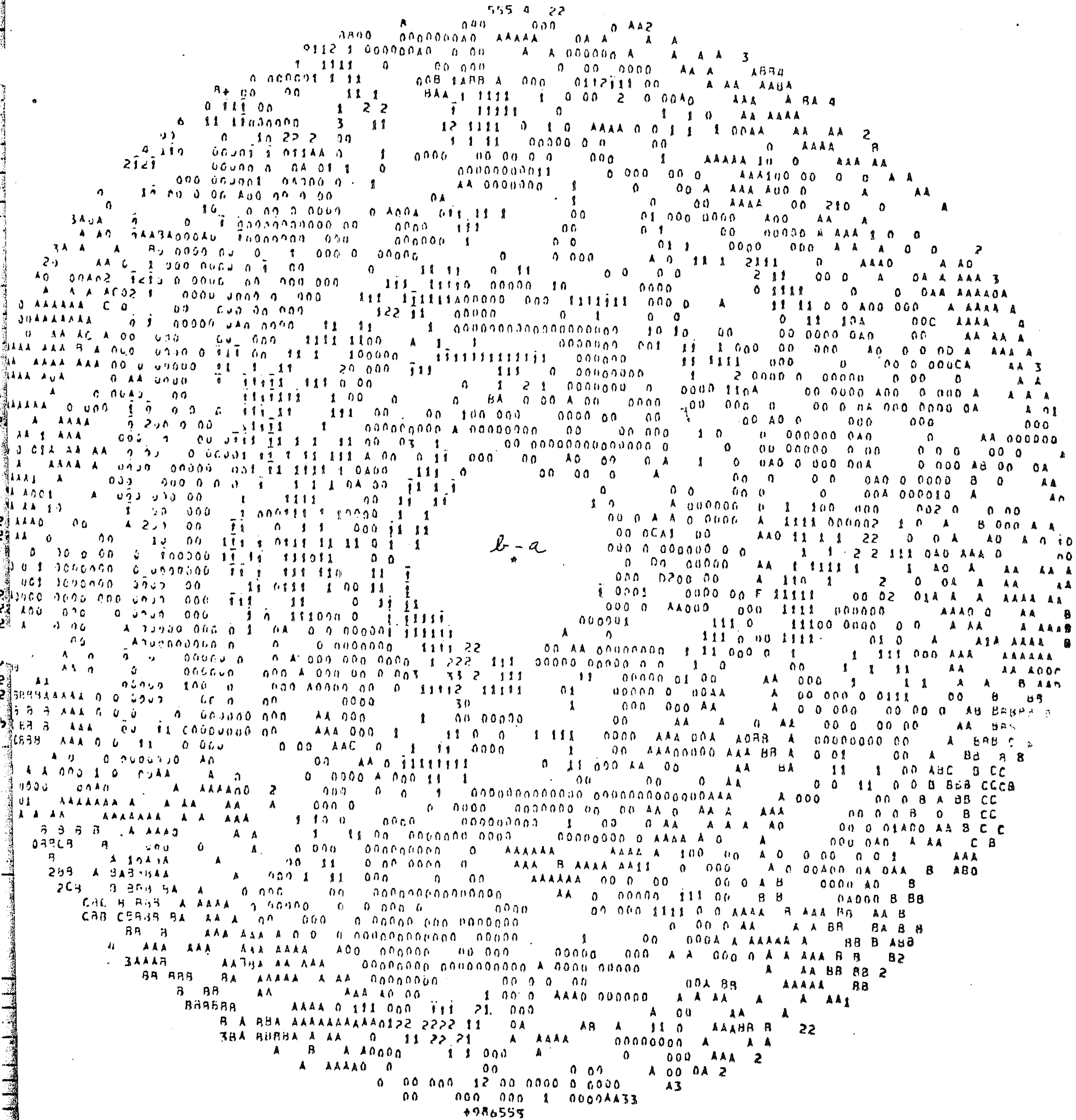
Figure 19: Difference map for 2nd DA/RA vs. 1st DA/RA. Here, the strongly affected areas have disappeared, i.e., there was no further change between the two DA/RA cycles. The effects were removed from the dish by readjustment of the panel-support differential screws. No similar problem was encountered with DISH 1, the first "production" dish.
