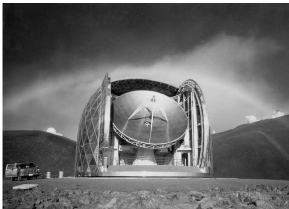
Figure 1: Unlike the OVRO Leighton telescopes which operate in open air, the CSO is housed in a dome.
